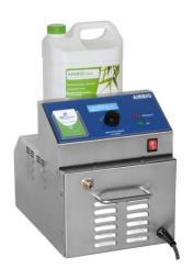
The AIRBIO/APABIO process enables an airborne disinfection of surfaces in rooms between 10 and 300 m3. The process is therefore based on two parts, the AIRBIO machine and the APABIO agent. The AIRBIO machine sprays the APABIO agent into the atmosphere thanks to compressed air. Then, a nozzle mixes and sprays the product in micro-droplets in order to overflow the whole romm to disinfect.
